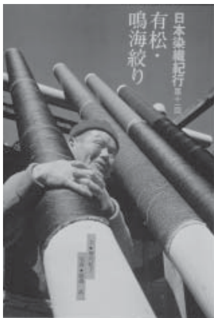
Mr. Reiichi Suzuki's father invented arashi shibori in 1880 in Arimatsu village by dyeing 4 yukata or summer kimono lengths of 14-inch wide cotton cloth on 13-foot wooden poles with indigo dyes. PVC poles are now used by contemporary artists instead of the traditional wooden poles.
