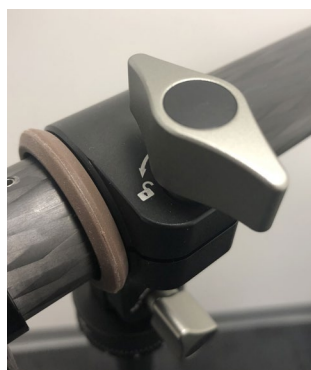
Image 27: Unlock dial on overhead arm to centre arm over tripod stand and lock in place.
