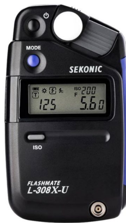
Image 17: Use a light meter to measure the lighting set-up. The aperture based on the current lighting is displayed in the bottom right corner.
