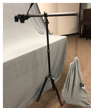
Image 28: Overhead photography set-up with attachment arm positioned over table. Use a sandbag and weights to balance the weight of the camera.
